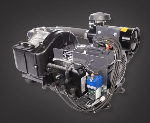
Our 24 VDC solutions are avalaible from 2.2 kW to 5.5kw, offering a airflow from 160l/mn to 525l/mn at 10 bar. The 24 VDC solutions are perfectly suitable for truck application, to supply air for the brake or the suspensions.
