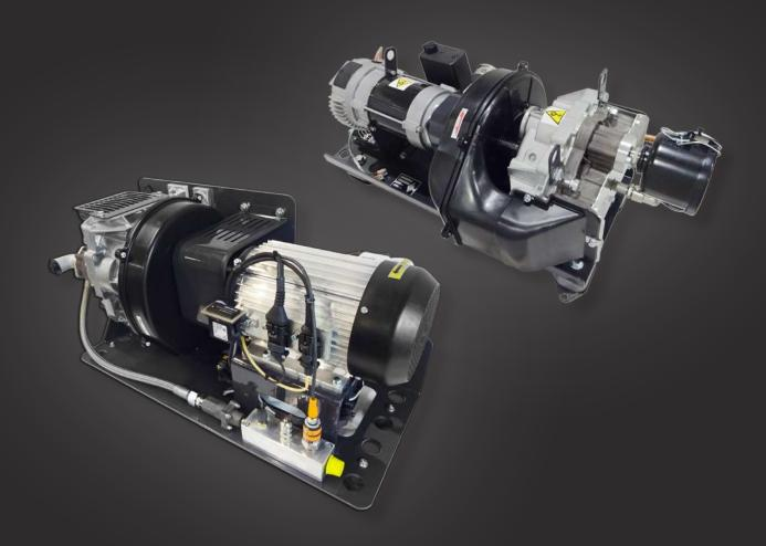
Our 48/80 VDC solutions are avalaible with 2 motors. The 80 VDC solution is powered by BLPM brushless motor delivering 1.5 kW. The 48 VDC solution is powered by the AMB motor, avalaible in 2.2kW and 3.7kW. The 48 VDC solutions are suitable for handling and the 80 VDC solutions is suitable for airport handling.
