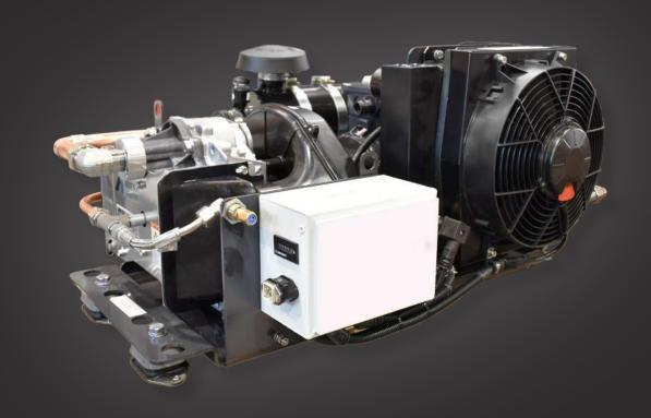
Our 400 VAC solutions are available with a range of motor going from 2.2 kW to 7.5 kW with a rotation speed of 3000 RPM and provide 240l/min to 640l/min at 10 bar. This solution is suitable for railway system and urbain railway system.
